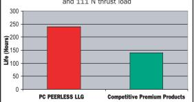
\* This test differentiates among wheel bearing greases having distinctly different high temperature characteristics. The longer the life, the better the protection.
